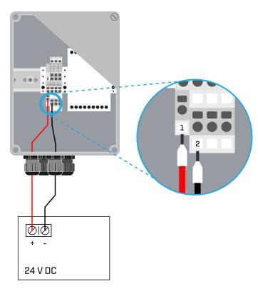
Fig. 2: Power supply connection
